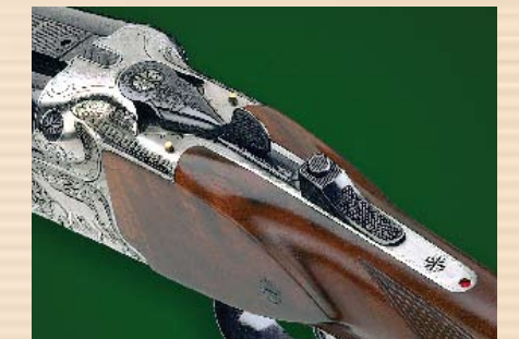
Three-position cocking slide in forward position: The locks for the upper barrels are cocked, the safety for the left barrel is off; the safety for the right barrel is on, the lock for the lower barrel is cocked and ready to shoot.
