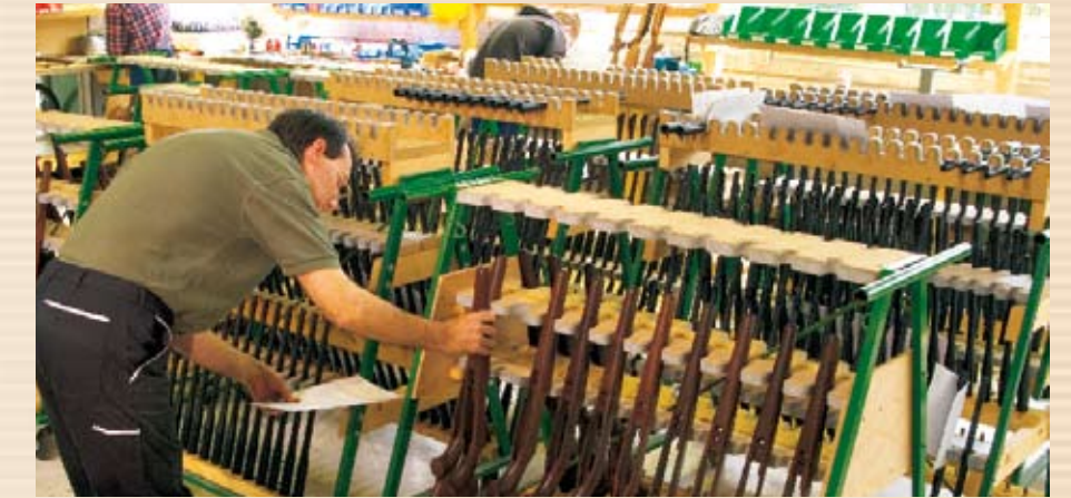
The components from the metal and wood-working shops are married in the assembly area.
