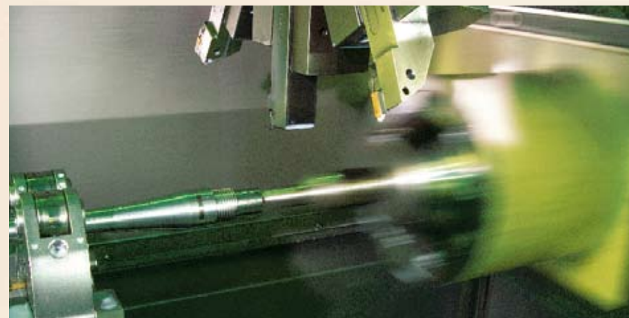
Steps on the road from round steel to barrel: The inside face of a forging is ground down until the surface roughness is less than 2µm. The actual cold forging and machining of the outer contours follows.
