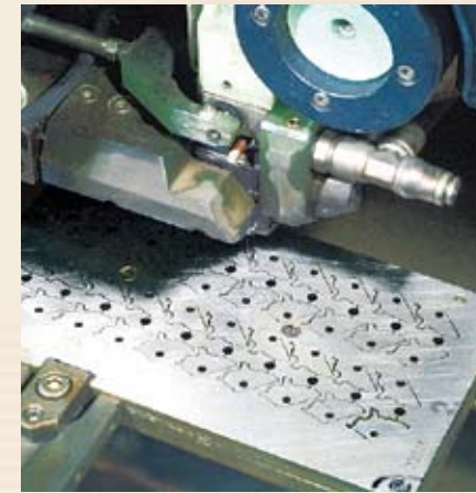
Electrical discharge machining makes it possible to mass produce small parts and complex shapes; for example, shaped openings in receivers.
