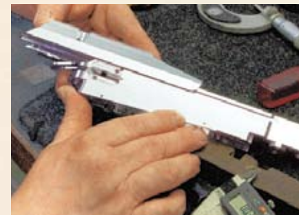
Precise integration: locking housing and action assembly on a KRI.
