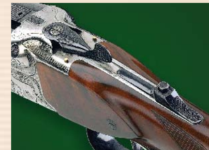
Three-position cocking slide in rear position: The locks for the upper barrels are cocked and the safety is on; the lock for the lower barrel is decocked.
