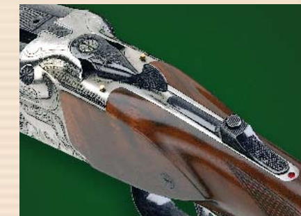
Three-position cocking slide in center position: The locks for the upper barrels are cocked and the safety is off; the lock for the lower barrel is decocked.
